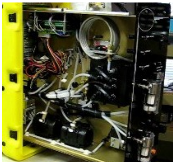
This image above shows the interior of a GeoStrata Technologies Eclipse Gas Chromatograph that runs continuously in three minute cycles. Two valves are used to switch the test gas into the sample loop. After filling the sample loop with test gas, the valves are switched again applying carrier gas pressure to the sample loop and forcing the sample through the Column for separation.
